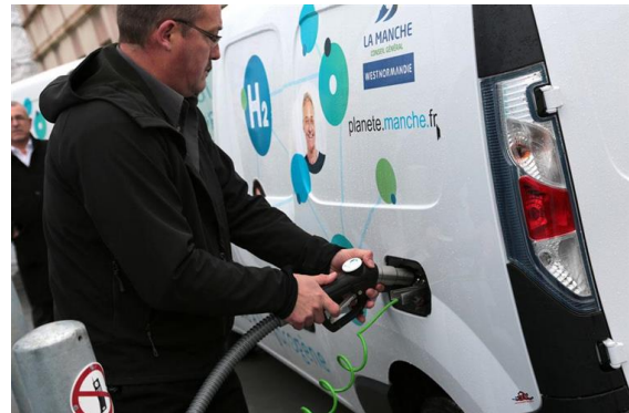
A Renault Kangoo Z.E.-H2 connected to the hydrogen refuelling station of the General Council of La Manche, in Saint
